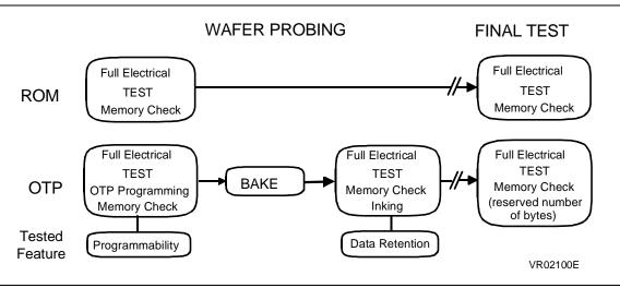
Although the programmability of the OTP die is verified as fully functional at probe test, the assembly process can **affect this parameter** in the finished product (for example by damaging some cells). It is therefore necessary to make a **final test** to check **programmability**. But since UV light cannot be used to restore OTP's programmed bytes once the die has been en-
