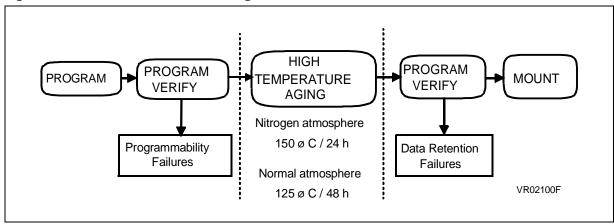
Screening devices that are subject to data retention failures will allow customers to obtain OTP devices with a similar quality level compared to ROM devices.
