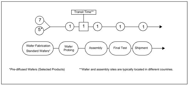
In order to limit lead time on ROM products, STMicroelectronics has introduced pre-diffusion technology on selected products. This allows a two weeks reduction in total cycle time. Also notice that MCU devices have to be ordered in specified minimum quantities for ROM version.
